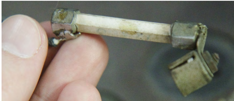
Figure 11: Non-RMA color coded 14,100 \Omega resistor.
