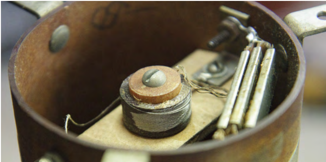
Figure 3: Altered concentrated coil located inside the PCRC.
