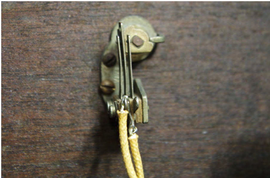
Figure 12: This two-position rotary tone switch was added by Termen.
