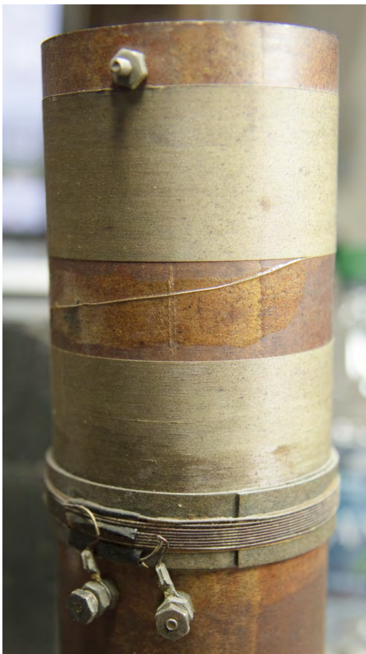
Figure 13: Volume coil with center windings removed and ends joined.
